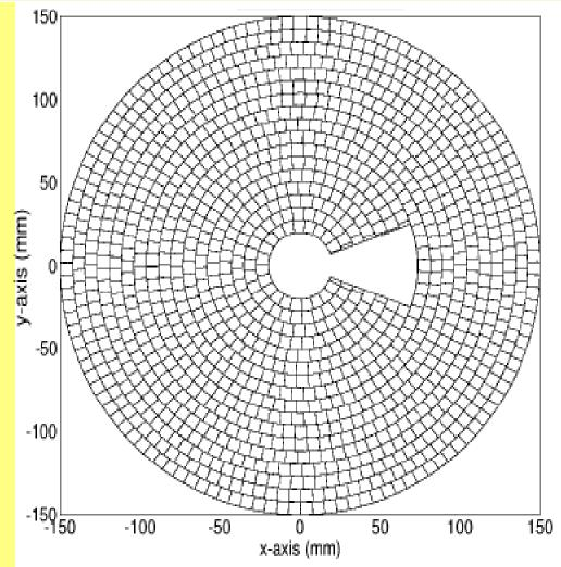
Cylinder: A palette extended through the depth of the BeamCal
