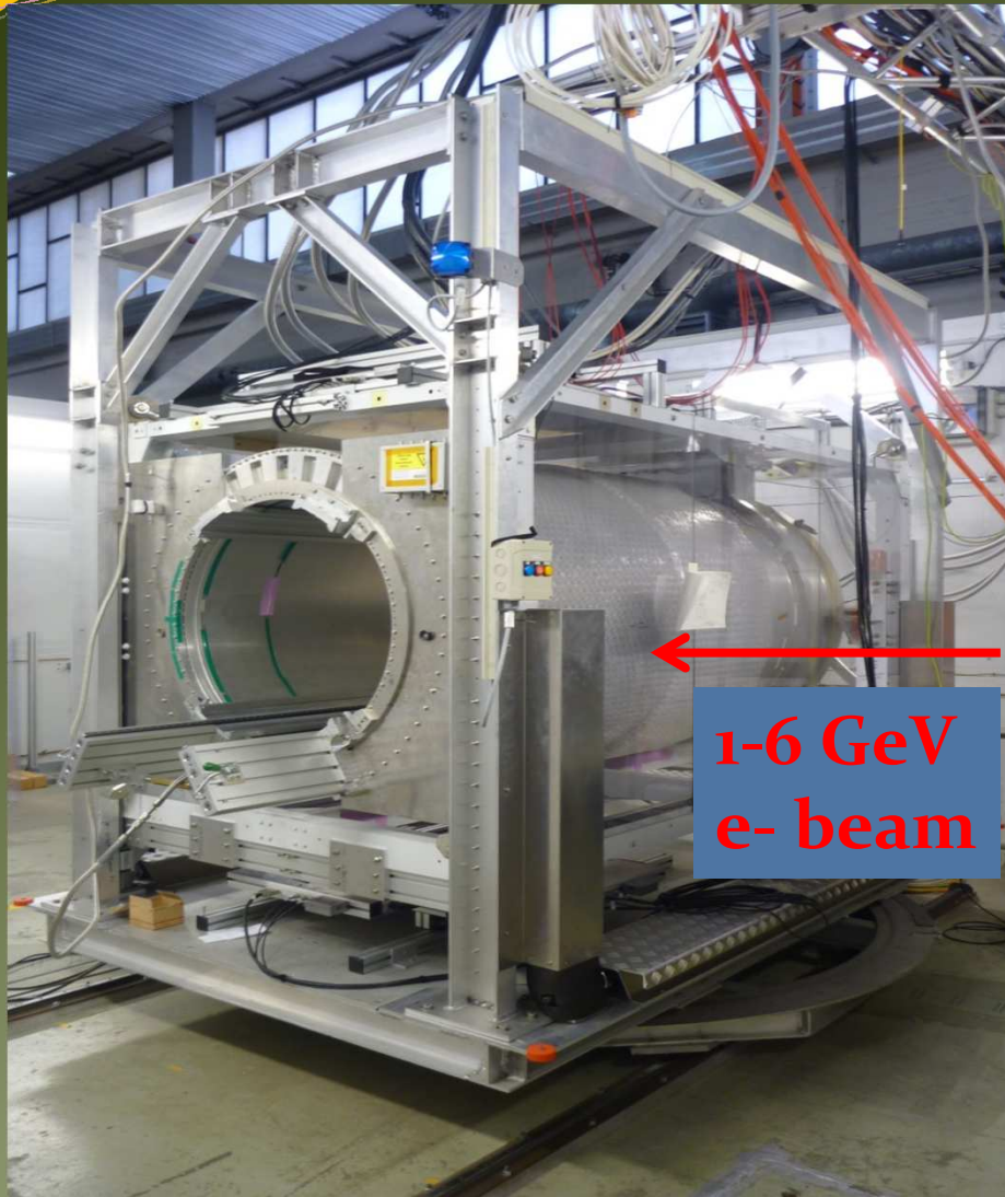
The movable stage and the 1T magnet.
