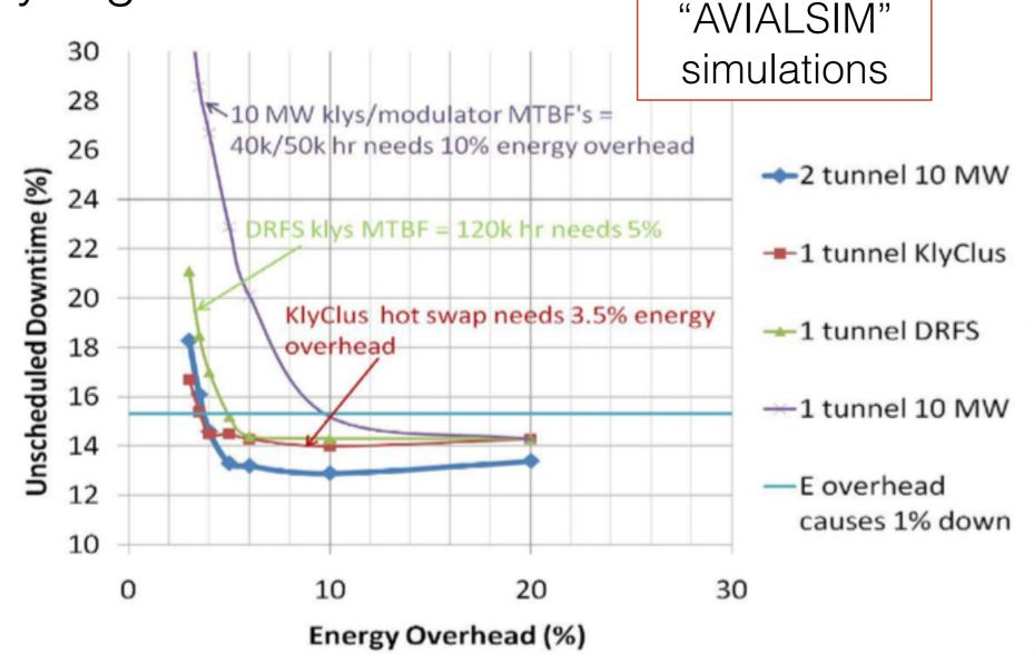
RDR/TDR: "two tunnels" cheaper than additional required linac overhead Klystron+modulator lifetimes now expected to be much higher (100k vs 40k hours)
