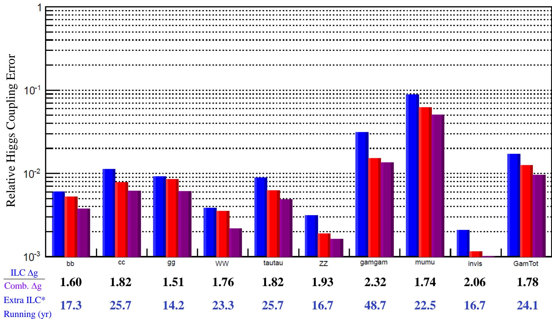
\*Additional ILC running required to match FCC-ee contribution to Combination. Assumes the same 1:2 luminosity ratio for 250:500 GeV except ZZ & invis which assumes all extra running at 250 GeV.
