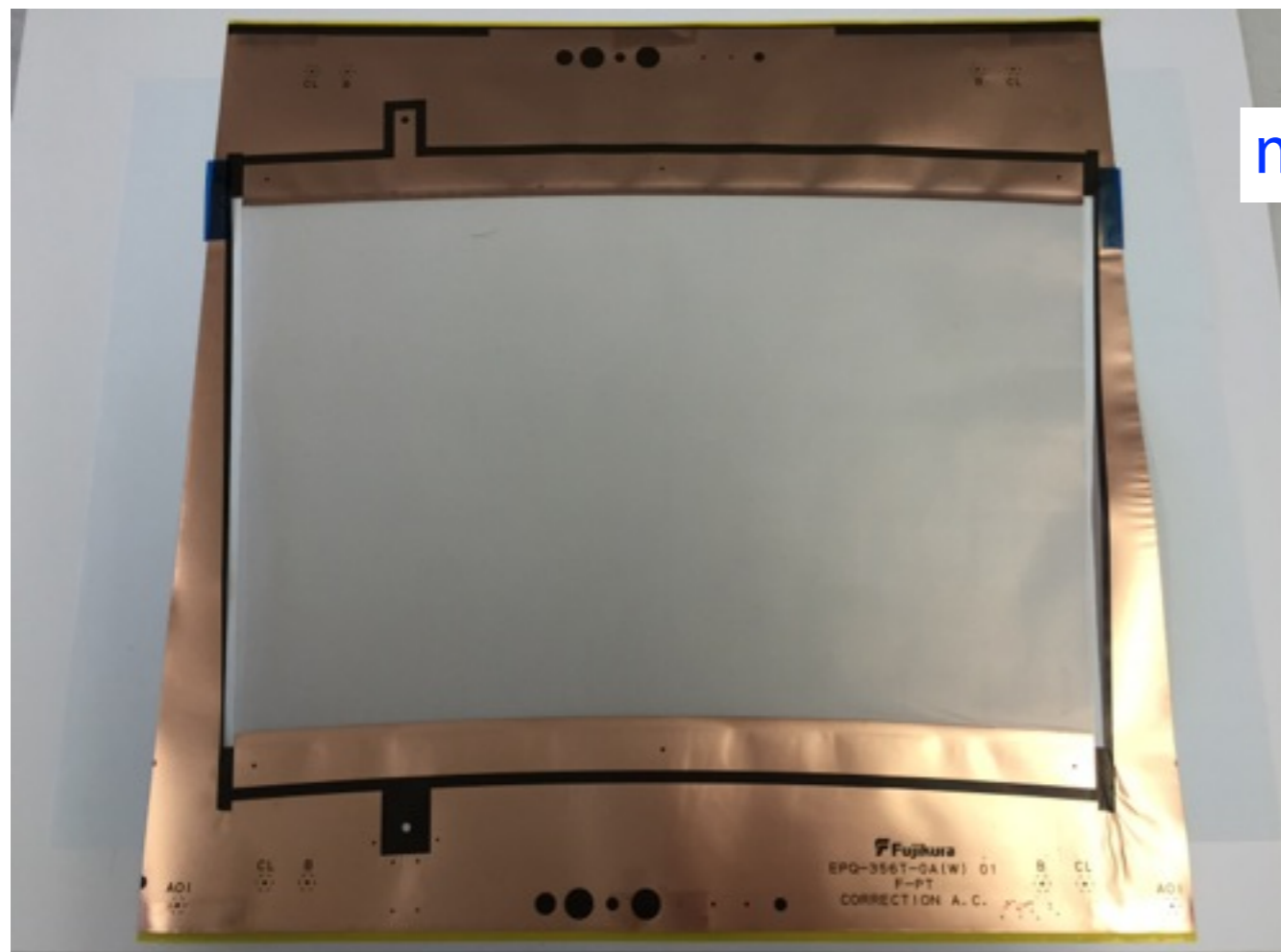
Large-aperture Gate-GEM (Fujikura Type 4 - 17 x 22 cm 2 )
