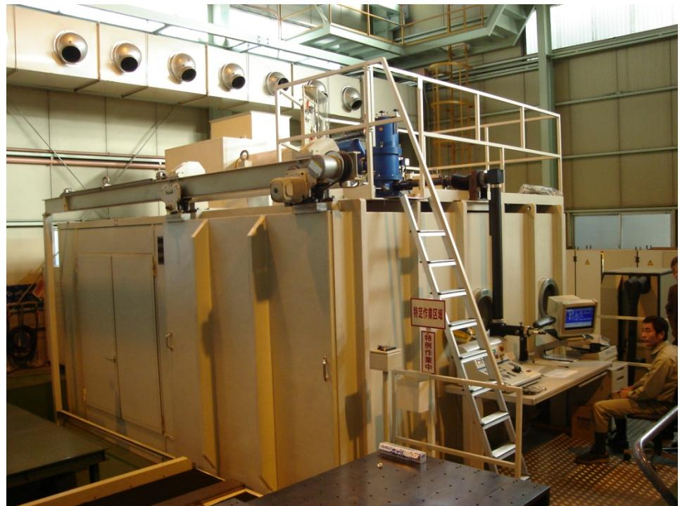
The chamber inside is pumped down to exclude the air before the EBW assembly.
