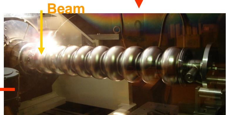
EBW of end-beam-pipes and cell-part
