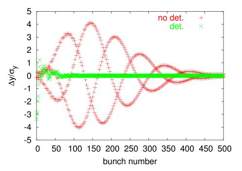
All main linac cavities are scattered by 500  $\mu m$
