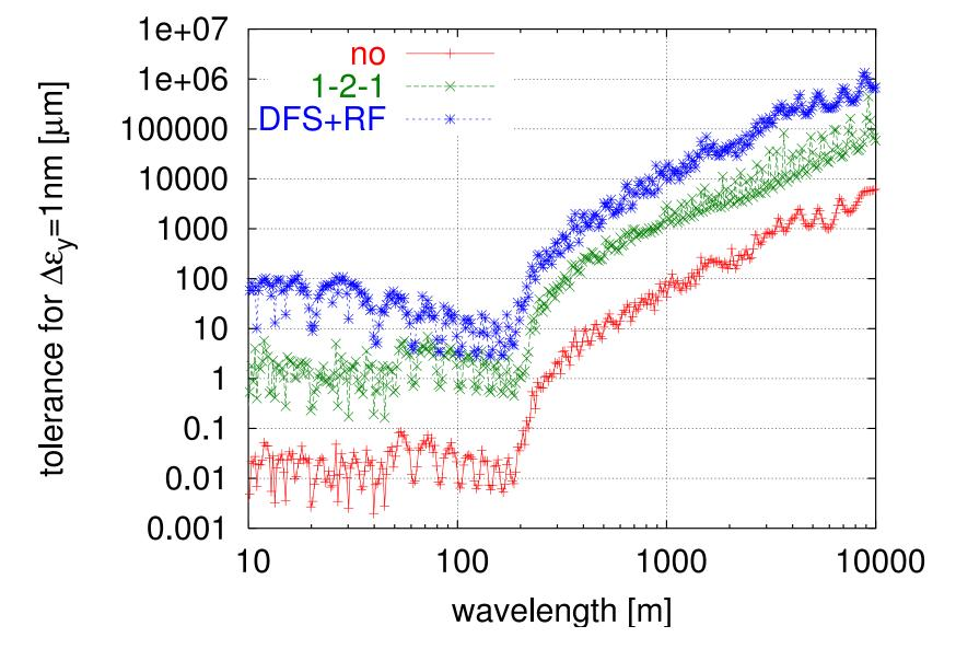
• Cosine-line misalignments, beta-functions clearly visible
