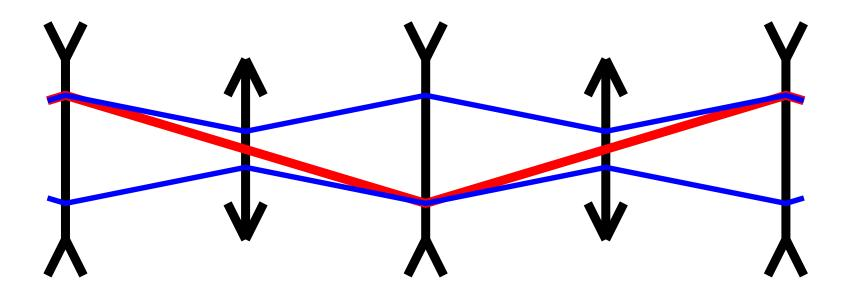
• Focusing is achieved by alternating focusing and defocusing quadrupoles
