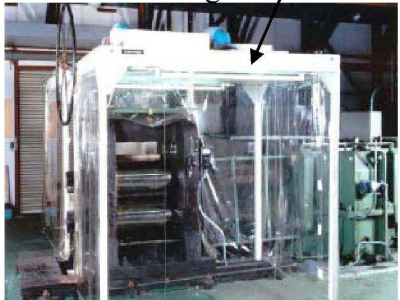
It is very important to avoid any contamination when rolling Nb plates.
