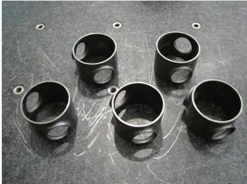
108 phi Nb Beam-pipe (pickup)
