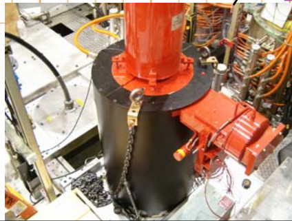
TH2104U Klystron (red) with Solenoid (black) Installed in an Oil Tank at ESB
