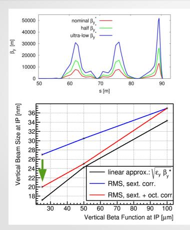
Decreased  $\beta_y^*$  causes the increase of  $\beta_y$  in the Final Focus region. In consequence the beam size is larger in the FF and more sensitive to beam line imperfections. It was checked that:
