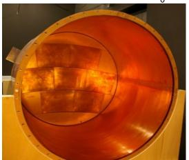
The endplate is able to host 7 readout modules (dimensions ~22x17 cm<sup>2</sup>)
