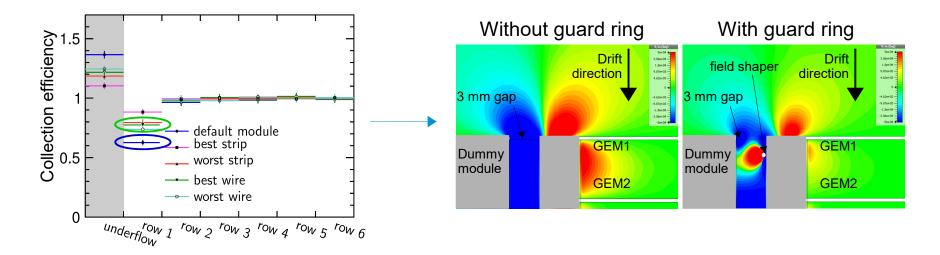
Loss of signal close to module edge partially recovered when introducing a guard ring
