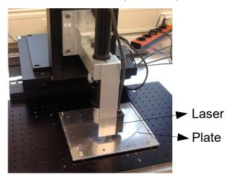
> Flatness of current GEM structure is at the level of 150 µm (rms)
