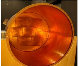
The endplate is able to host 7 readout modules (dimensions ~22x17 cm²)
