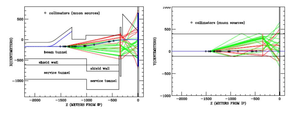
Muon trajectories the horizontal and vertical planes which hit a 6.5m radius detector for the condition of 5m long magnetized spoilers with a 1m gap at the right wall of the tunnel and a 1m gap at the top of the tunnel.
