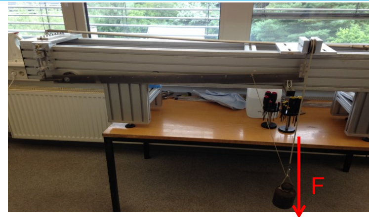
Tensile test setup of screw and insert shown Torlon screws
