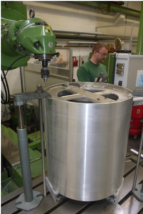
Mandrel during machining
