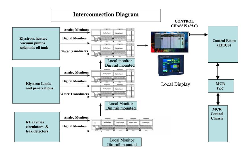
Monitors are commercial off the shelf equipment mounted near equipment with serial link to PLC
