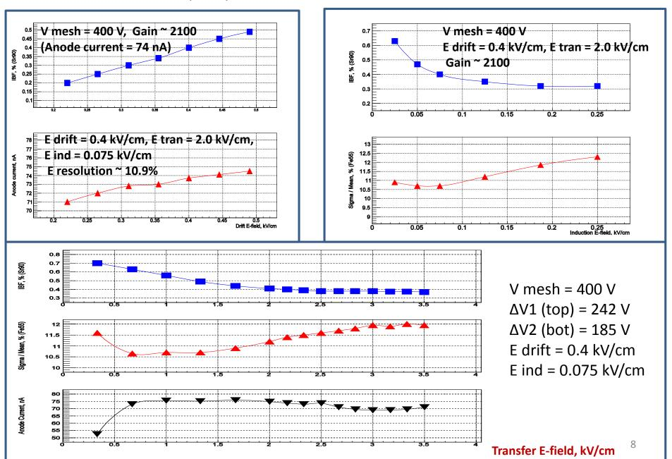
Energy resolution (Sigma/Mean for <sup>55</sup>Fe) vs. ion backflow (IBF) for various gas mixtures and different MMG and GEMs voltages.
