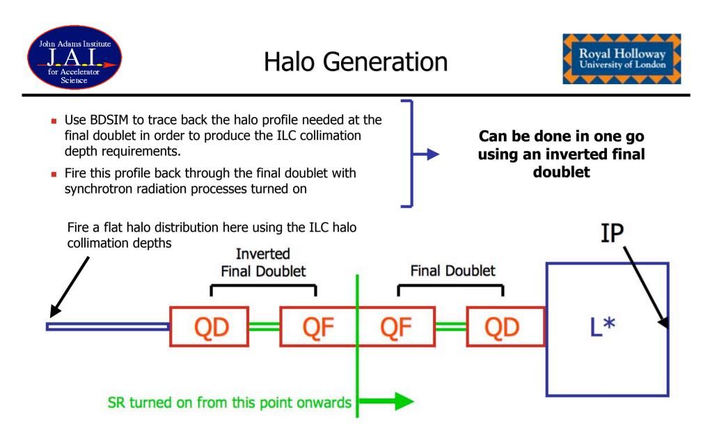
• Of course, BDSIM could have created the Halo distribution by tracking the electrons from the Linac down the entire Beam Delivery System.
