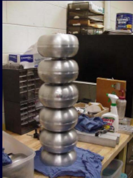
Tuning and HOM damping measurements at DESY
