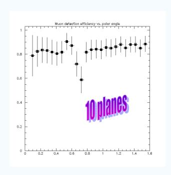
Single μ detection efficiency vs. polar angle
