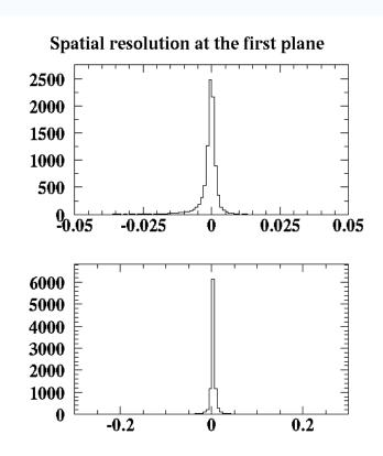
$\theta$  and  $\phi$  r.m.s. at the first detector plane.
