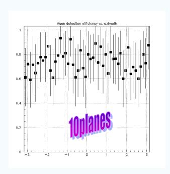
Single μ detection efficiency vs. azimuth
