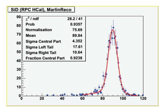
example: ZO reconstrution, full PFLOW implementation MARLIN package (LDC) applied to the SiD detector
