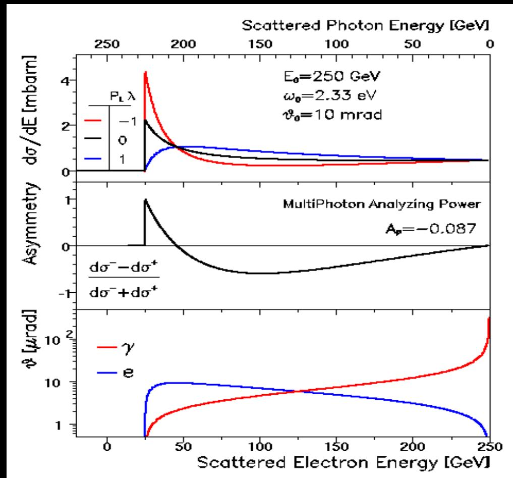
$$\frac{d\sigma}{dy} = \frac{2\sigma_0}{x} \left[ \frac{1}{1-y} + 1 - y - 4r(1-r) + P\lambda rx(1-2r)(2-y) \right]$$
