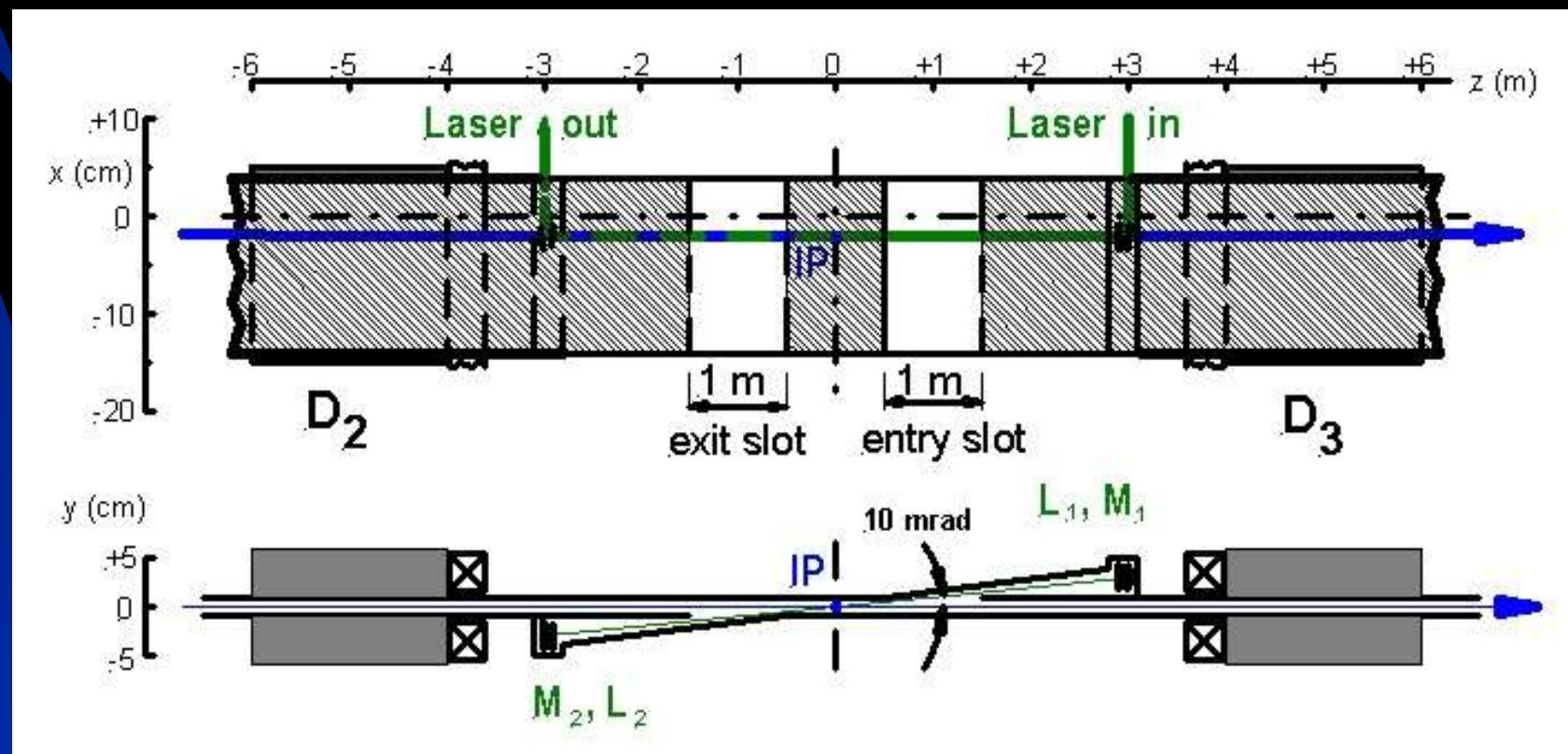
laser beam crossing requires  $\sim 1$  m long insertion/exit slots along  $z$
