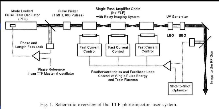
Fig. 1. Schematic overview of the TTF photoinjector laser system.
