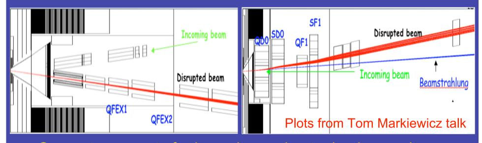
Separate magnets for incoming and outgoing beams in 20mrad extraction
