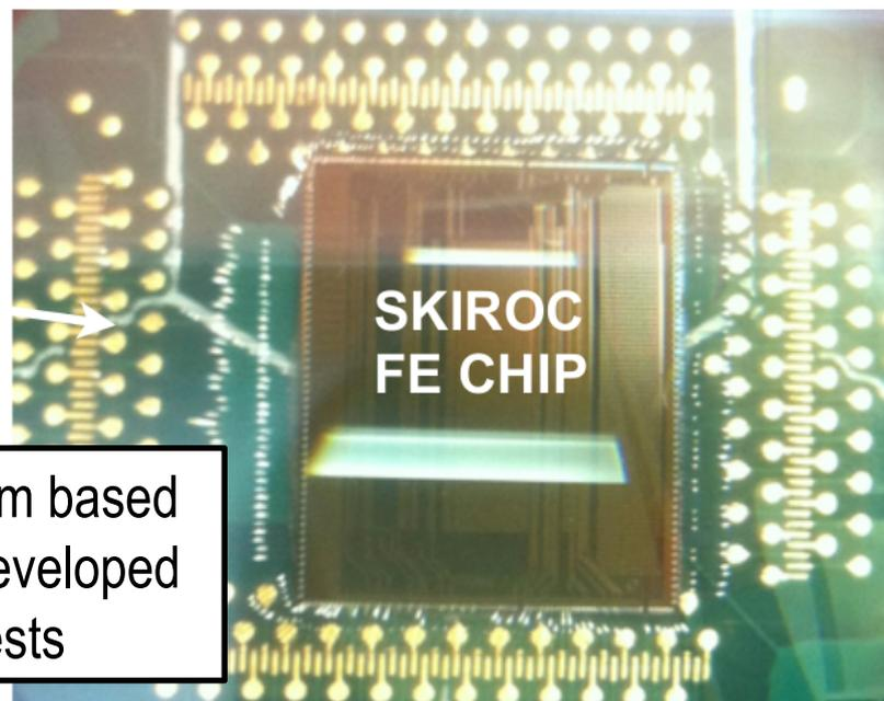
CMS initial testbeam based on SKIROC chip developed for CALICE tests
