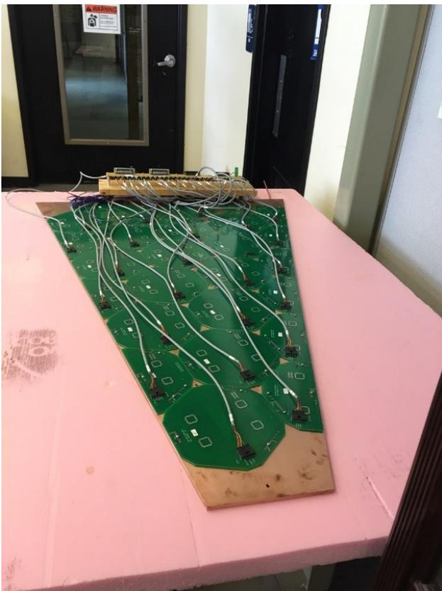
“dummy” cassette for thermal tests
