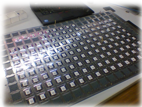
Original system: SiPM + Tile
