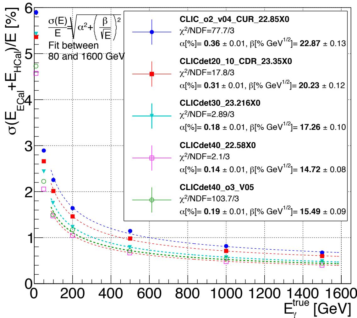
Additional material leads to a slightly higher resolution than with the original 40 layer assumption, still performs better than 30 layer options (both with constant and non constant sampling) over whole range
