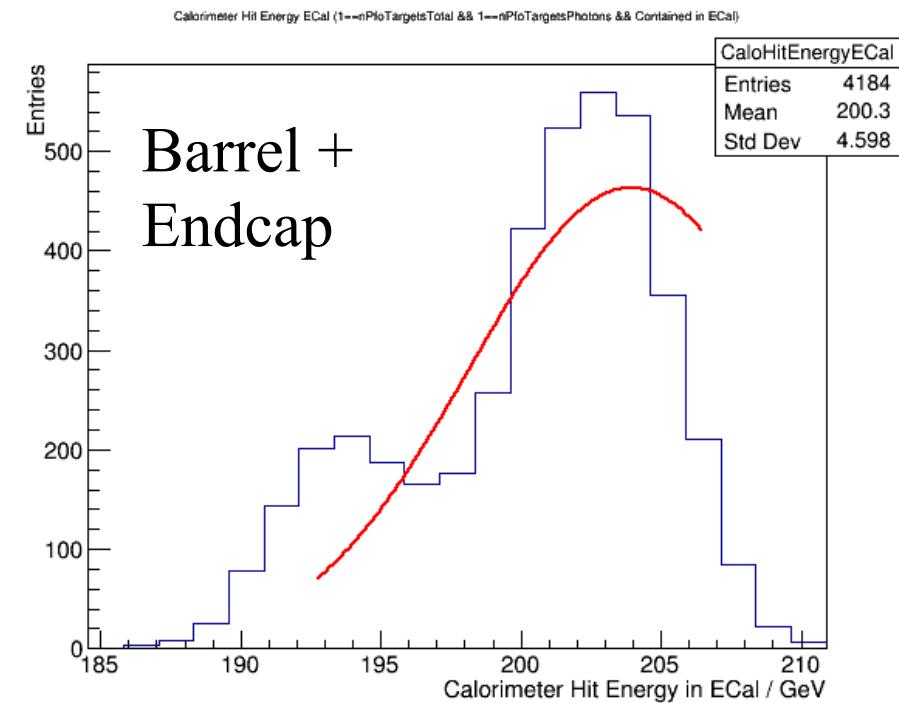
Use values from samples up to 200 GeV, for Barrel and EndCap mix two peaks start to appear, due to different behavior of energy contribution from HCAL
