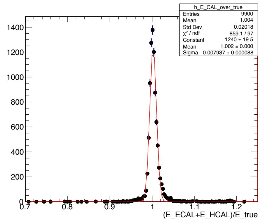
Different HadToEM scale needed for HCAL energy contribution in barrel and endcap: recovers scale behavior
