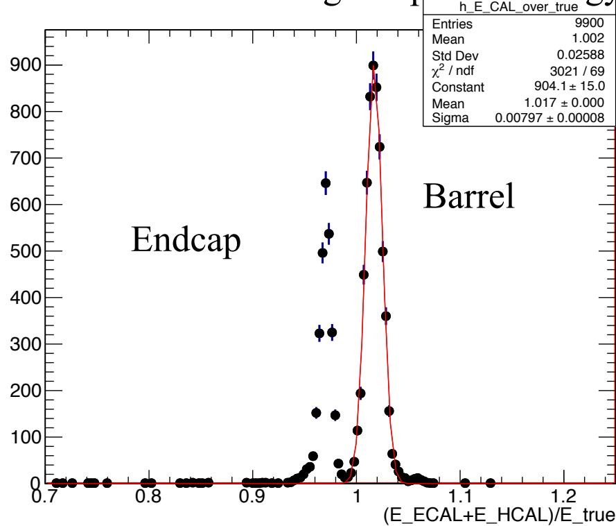
Default calibration constants: clear two peak, higher peak barrel, lower peak endcap
