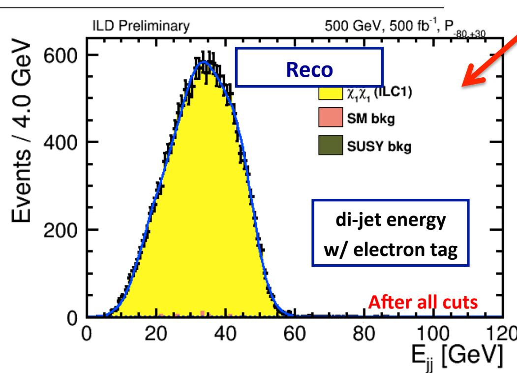
Change in distribution of Di-jet energy with respect to cuts (SIGNAL)
