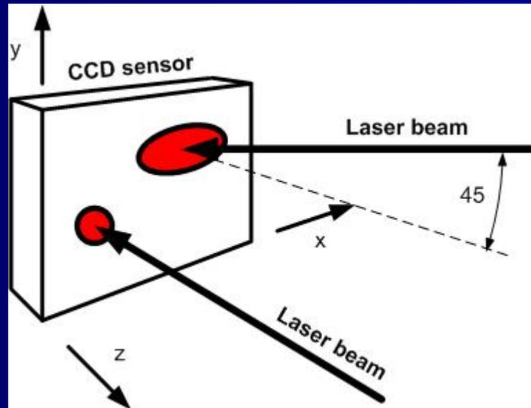
Two laser beams (one perpendicular, second with  $45^\circ$  angle to the sensor plane) allows us to measure XYZ translation in one sensor
