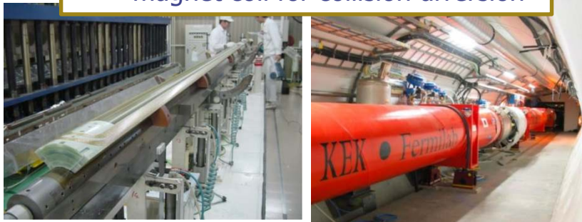
LHC: Superconductive 4 pole magnet coil for collision diversion
