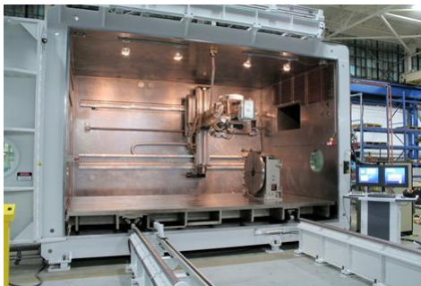
Electron beam welding in big vacuum chamber Tribute to SCHIAKY
