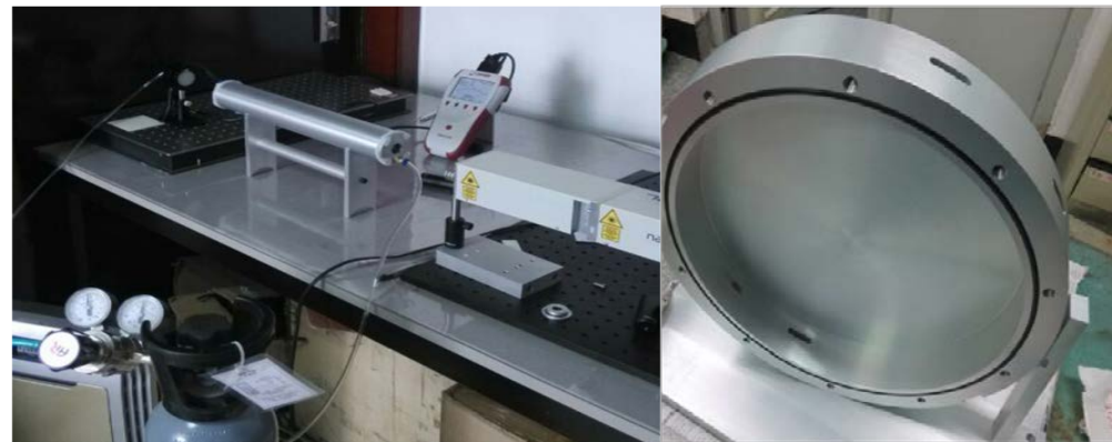
The assembled module test with 266nm laser
