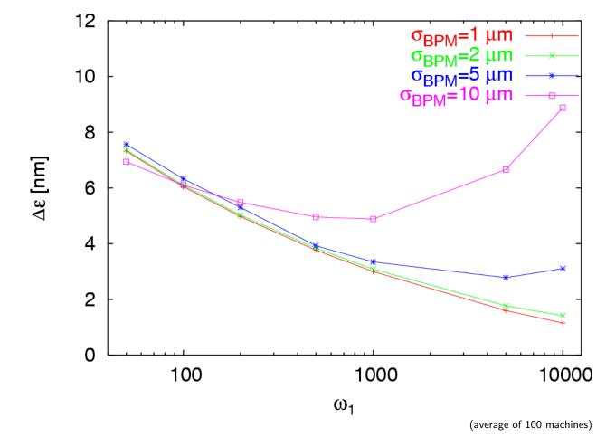
for a laser-straight linac, DFS (with  $\omega$  "big", BPM resolution of 1  $\mu m)$  leads to excellent results but...
