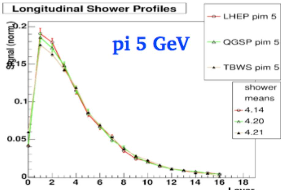
*LHEP and QGSP show good agreement with test beam data at low and intermediate energies*
