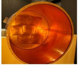
The endplate is able to host 7 readout modules (dimensions ~22x17 cm<sup>2</sup>)
