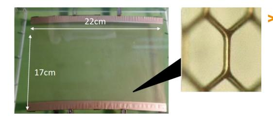
• Gating GEM provides high transparency for drift electrons (~85%) and should provide high blocking power for positive ions (10<sup>-4</sup>)
