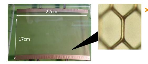
• Gating GEM provides high transparency for drift electrons (~85%) and should provide high blocking power for positive ions (10<sup>-4</sup>)
