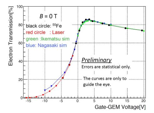
Electron transmission rate measurements and simulations
