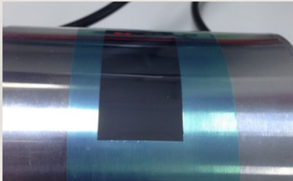
50µm thick silicon sample (20x50mm held on a vacuum jig; r=45mm)
