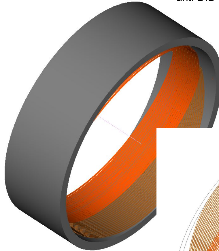
Direct wind scheme anti-DID inside main solenoid
