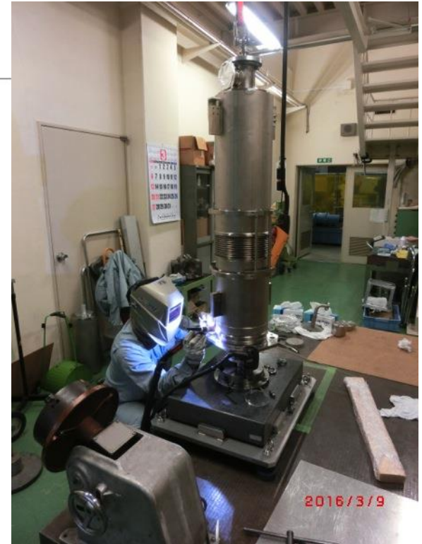
TIG welding He tank with cavity
