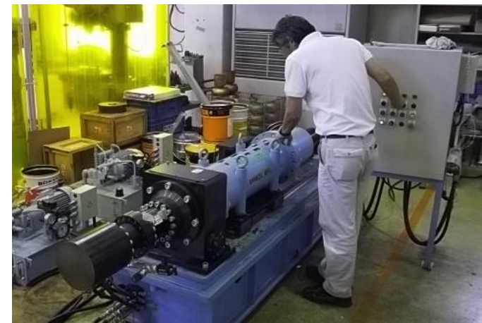
Hydroforming machine (Final hydraulic pressure: 25 MPa)
