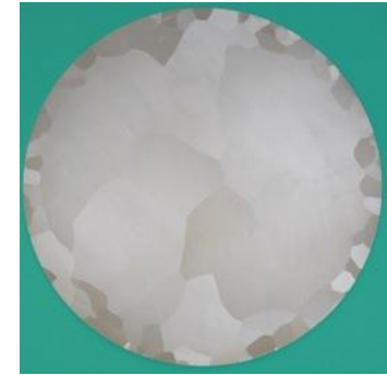
Ingot sliced Niobium (Tokyo Denkai) (Dia: 260 mm)
