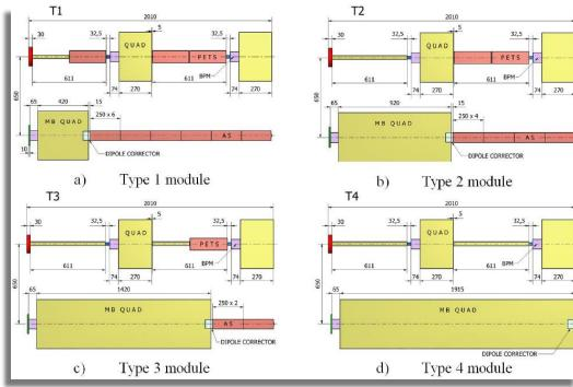
Studies looking at the <u>Main Beam Quadrupole stabilization</u> problem have shown that an independent support is required to guarantee the level of stability requested by the challenging beam dynamics.
