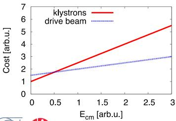
With the increase of the klystron and modulator efficiencies, the interest for a low energy stage driven by klystrons is growing.
