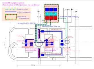
• To prevent the complexity around packman, 2K refrigerator had better be installed at the dedicated cavern in the each accelerator side which is very close to CC and QF1 as shown in above figure.
