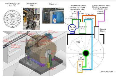
Most of the cryo-equipment should be located on the YB0 platform in order that ILD detector should be divided into 5 sectors as easy as possible.
