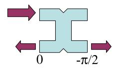
For cavity phasing:  $-\frac{\pi}{2} - \beta(P - h_H) = -k_0 P + 2n\pi$
