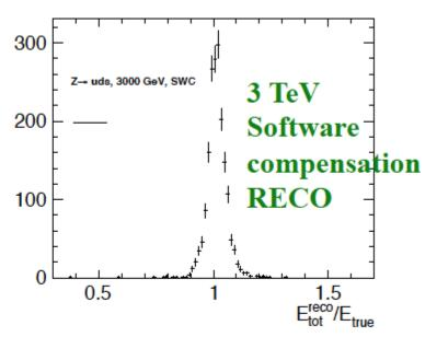
This behavior is gone with the software compensation (MHHHE removed), mean of reconstructed energy distribution within 1 % of true energy for all energy points considered, symmetric distribution
