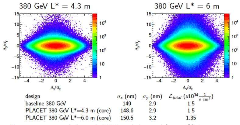
Beam transported through BDS with larger L\* is 10% bigger in vertical direction which compromise reaching the total luminosity goal at this energy stage
