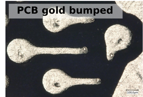
Gold Ball-wedge wire-bonding
