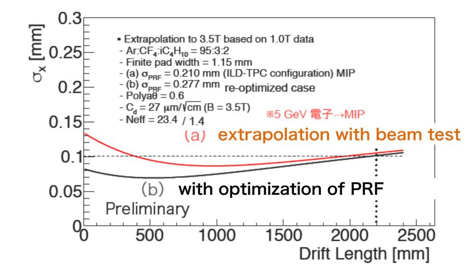
>80% Gate + GEM system can provide required performance at ILC
