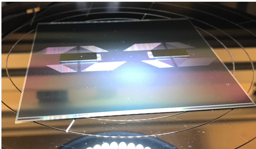
Fig.: Bump Bonded Sensor on the probe station
