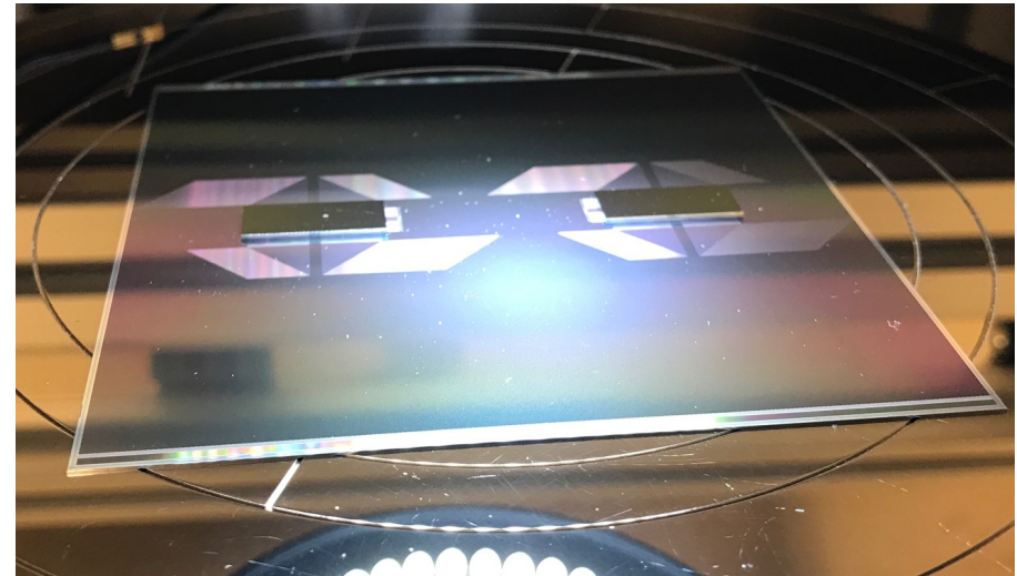
Fig.: Sensor with bump bonded KPix on the probe station
