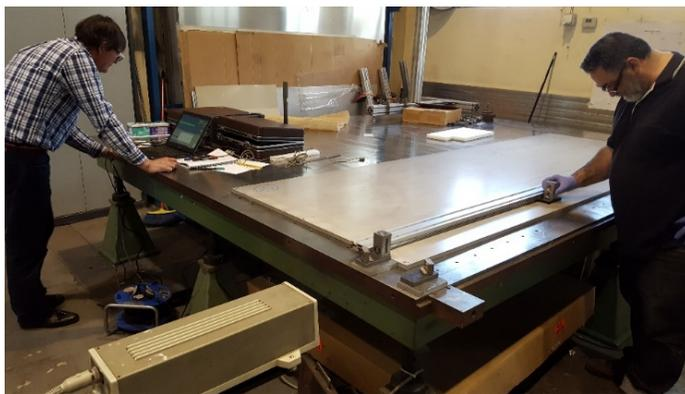
Measurements using **laser interferometer**.
