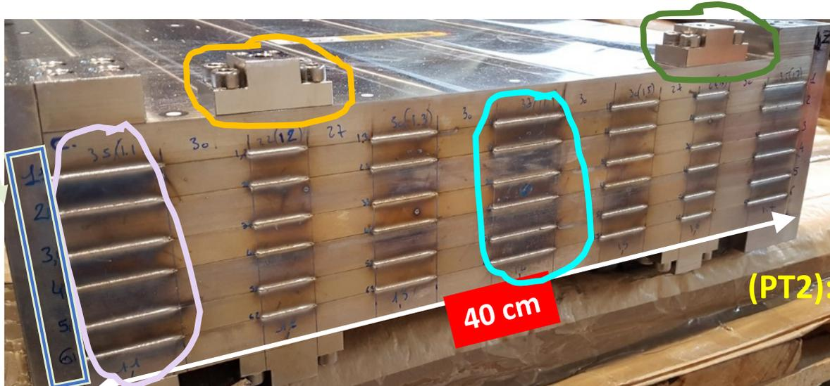
The welding is performed in a certain order not sequential, “jumping” in between the different welding point positions (horizontally and vertically).
