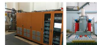
Fig. 8: L band Marx Modulator and ILC 10MW klystron
