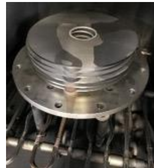
Electron beam welding of end-cell
