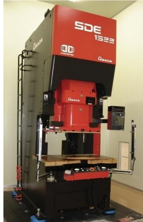
Servo press machine (AMADA, Japan) Max. applying force: 1500 kN
