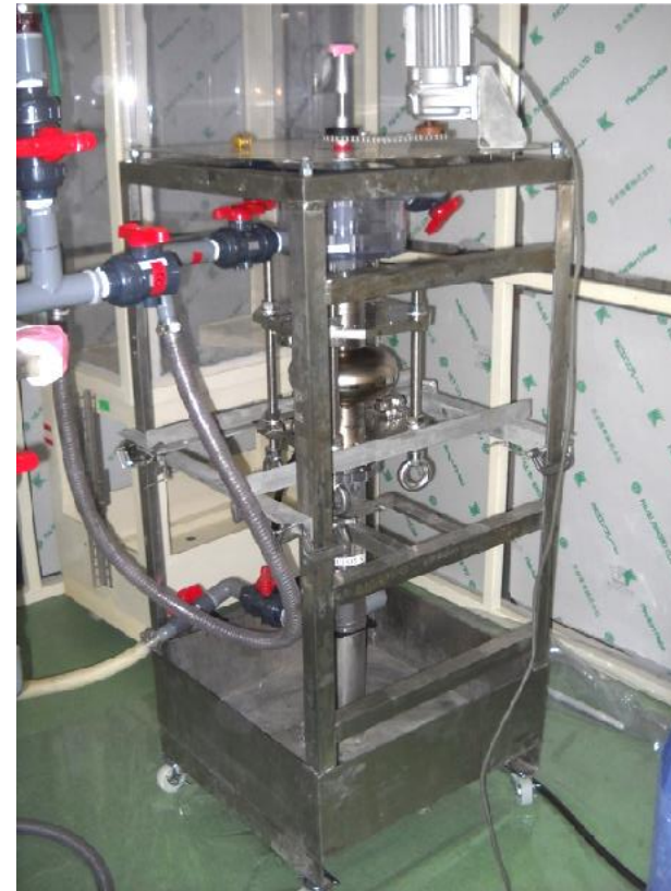
VEP Stand for Single Cell Cavity
