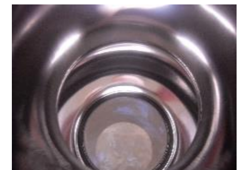
Cavity Surface after VEP-1
