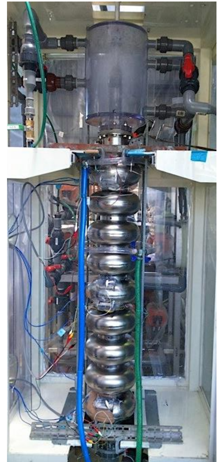
Coupon Cavity at VEP Stand
