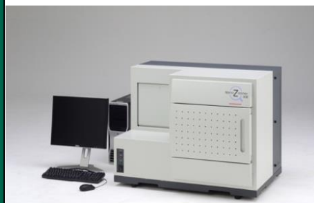
NanoZoomer-XR (Process up to 320 slides automatically)
