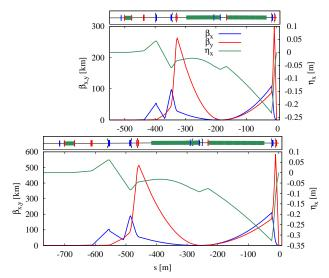
$\blacksquare$  A scan of the dispersion profile has been performed in order to optimize the luminosity for both  $L^*$  options
