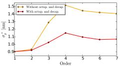
Vertical beam size  $\sigma_y^*$  reduced from 1.4 nm to 1.07 nm by using octupoles and a decapole at the appropriate locations
