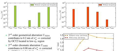
Vertical beam size  $\sigma_y^*$  reduced from 1.4 nm to 1.07 nm by using octupoles and a decapole at the appropriate locations
