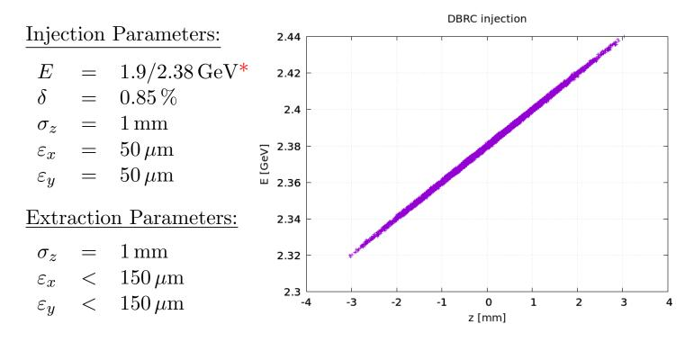
\* The DB energy is 1.9 GeV for CLIC's 1st stage and 2.38 GeV for stages 2 and 3. Most optical properties of the lattice are similar.
