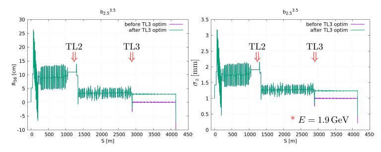
The decrease in bunch length originates in non-zero  $R_{56}$ (unwanted side-effect of previous optimisation scans) TL3 has already been optimised to have  $R_{56} \sim 0$ TL2 is next...
